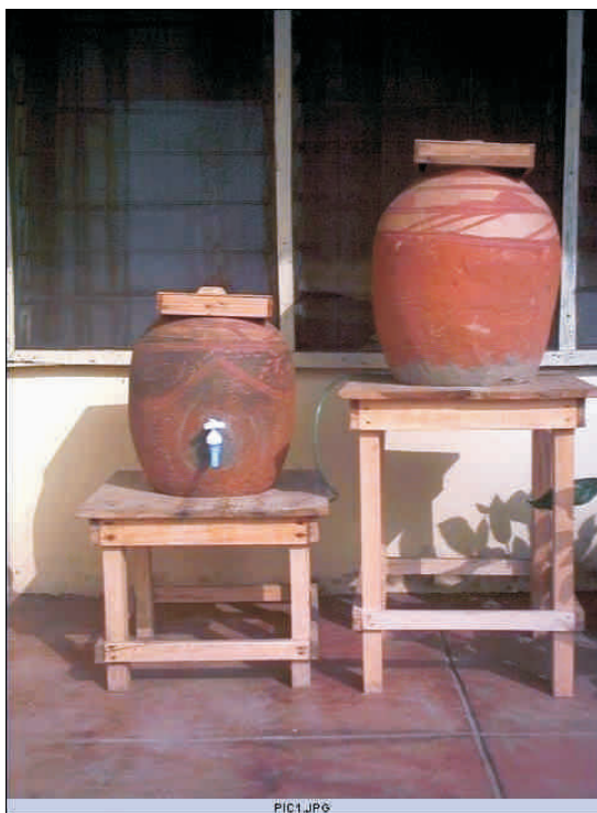
Figure 4: Earthenware sand water filter (Twin pot, downward flow)
