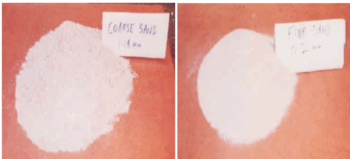
Figure 2: Size of fine and coarse sand used for constructing the sand water filter
